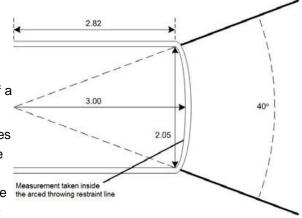
• The center of the circle is the point for the measurement and shall be marked. The sector is 40°.
